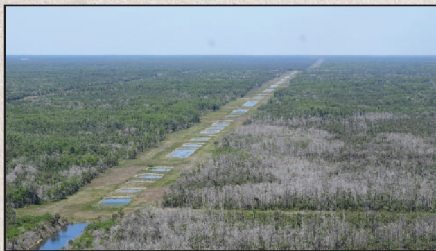
Plugging canals a part of restoring natural sheet flow in Picayune Strand
